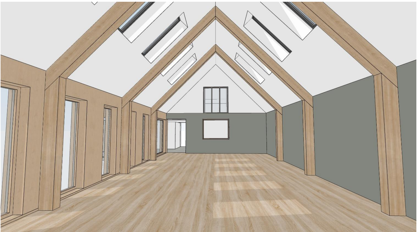
Above: the main hall showing exposed timber glulam trusses, entry door, serving access & first floor viewing gallery window.
